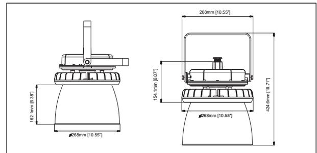
This structure can make the lighting distribution more concentrated for special beam angle.
